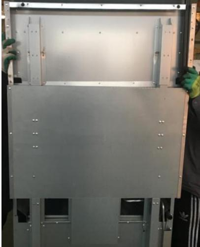
3. Screw the 12 screw holes with self tapping screw.
