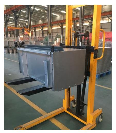
2. Lift the Salamander boiler and let the back support beam come through the range back support beam.
